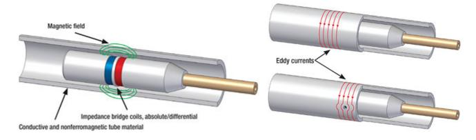
Two coils are excited with an electrical current, producing a magnetic field around them. The magnetic fields penetrate the tube material and generate opposing alternating currents in the material. These currents are called eddy currents.
